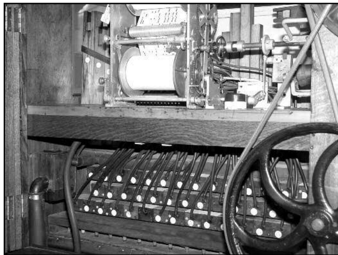
Figure 4. A rear view details the back of the Artizan A organ. Note the pressure roller sitting on top of the tracker bar. This is a feature retained from the original Artizan organ even though the organ has been converted to play from Wurlitzer Style 125 music.
